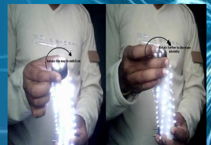
Figure 6: On-Off Arrangement of LED-Lamp
