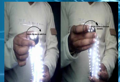
Figure 6: On-Off Arrangement of LED-Lamp
